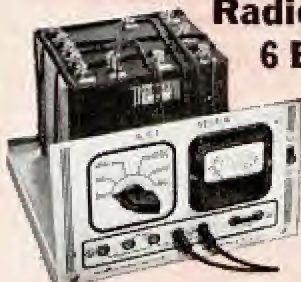
MEASURING INSTRUMENT (above) you build early in Course. Use it in practical Radio work to make EXTRA money. Vacuum tube voltmeter and multimeter. Measures A. C., D. C. volts, D. C. currents, Resistance, Receiver output.
